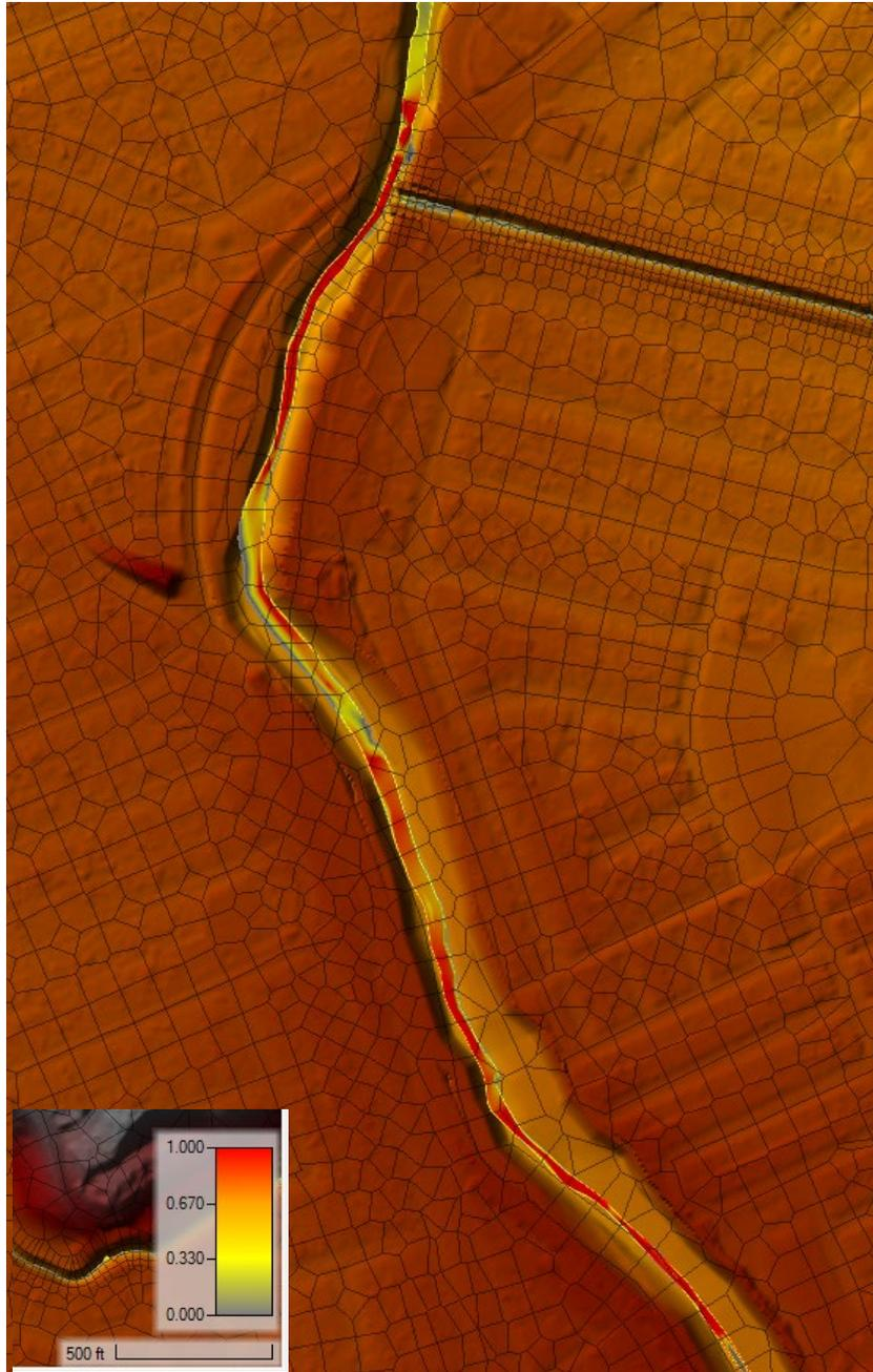
*Figure 11: Screenshot of RASMapper showing the Spawning HSI raster calculated using the HSI code in RASter Calculator. Legend displays raw HSI values.*
