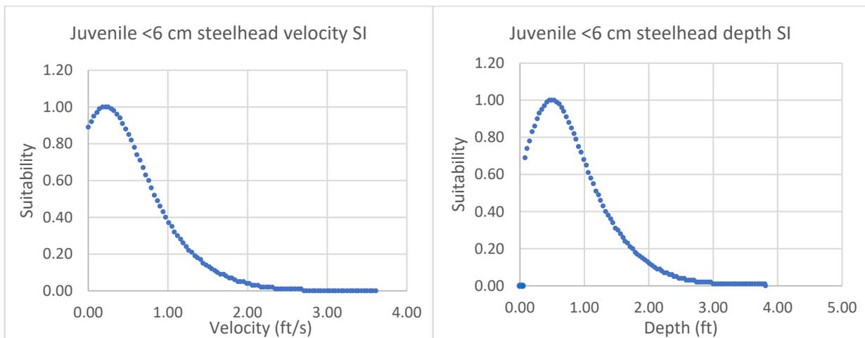
Figure 3. Left, Juvenile <6 cm steelhead velocity HSI curve. Right, Juvenile <6 cm depth HSI curve (Figures 122 and 123, respectively, from Holmes et al. 2014).
