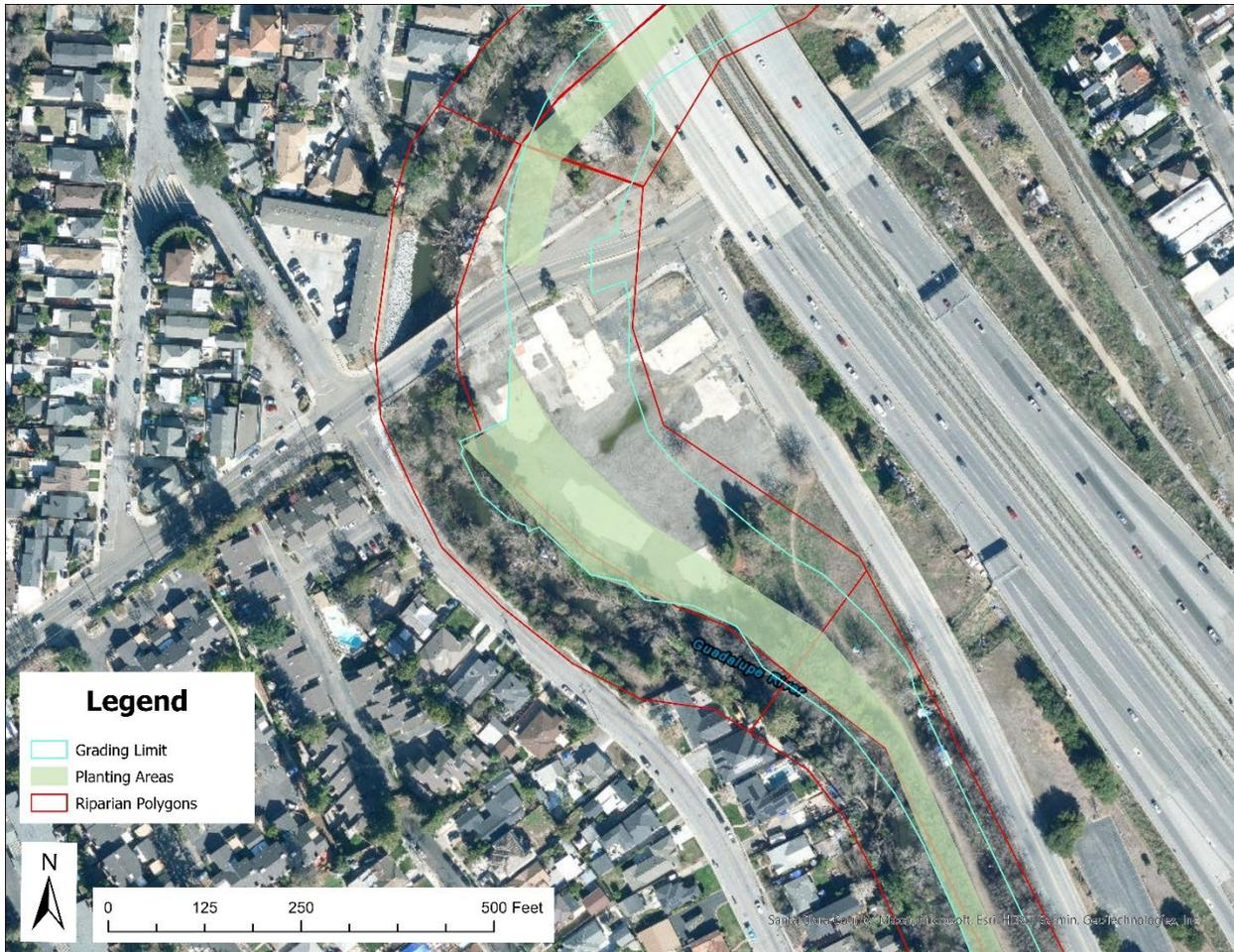
*Figure 7. Combination plan planting polygons (olive) shown with evaluation areas (red outline) and Combination plan grading footprint (light blue).*
