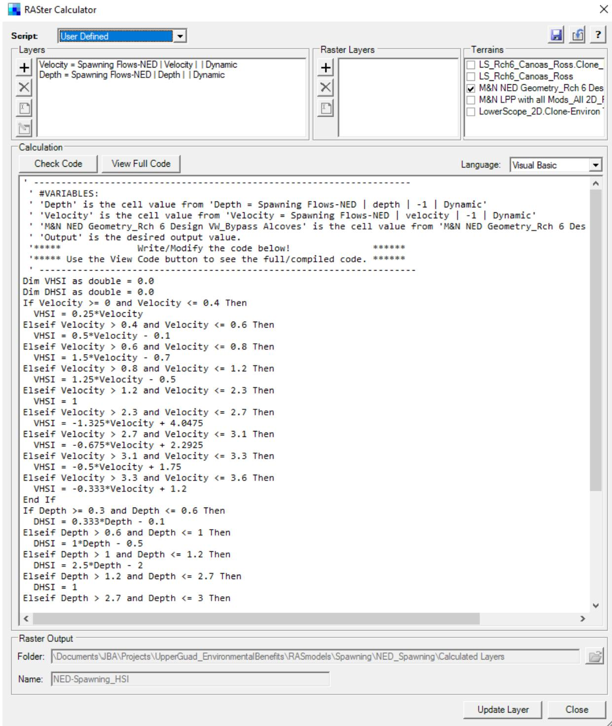
Figure 10: Screenshot of code for calculating Spawning HSI in the RASter Calculator interface.
