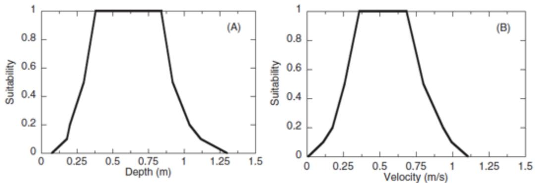
Figure 2. Spawning habitat suitability for velocity and depth in the Lower Yuba River, reprinted from Figure 3 in Kammel et al 2016.
