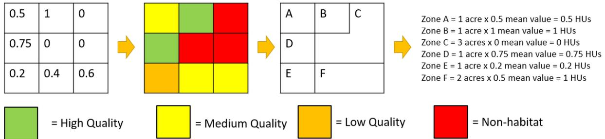
Figure 4. Schematic of GIS workflow to process habitat suitability rasters. In the first grid, the values are combined HSI values for each cell, and each cell represents one acre.
